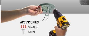
3.Connect supply wires to wires on fixture/bracket with wire nuts. Attach white to white, black to black, and copper wire to green wire as grounding connection, select lamp color desired with the CCT switch, see Fig3.
