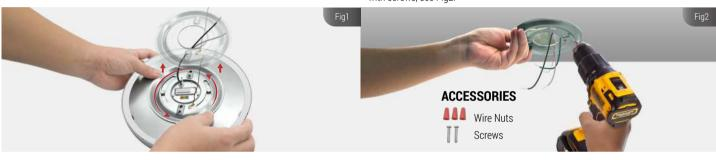
3. Connect supply wires to wires on fixture/bracket with wire nuts. Attach white to white, black to black, and copper wire to green wire as grounding connection, select lamp color desired with the CCT switch, see Fig3.
